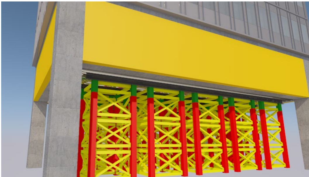
Figure 10 Using heavy-duty falsework system to support the single thick layer cast-in-situ transfer slab
